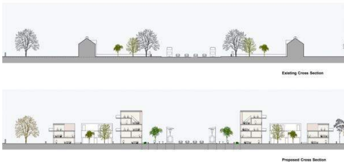
Figure 4: cross-section of the N11 before and after redevelopment. The existing houses and their surrounding land have been replaced by apartment buildings arranged around courtyards for high-quality family living and creating an urban boulevard whose buildings proudly embrace the street. The road has been narrowed to 40m, freeing up additional land for redevelopment while greatly increasing its capacity to transport people without reducing capacity for private cars compared with current levels.
